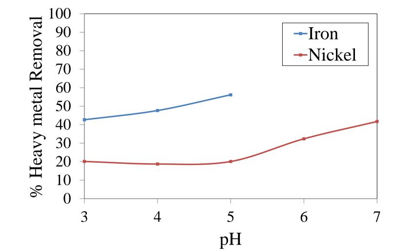
This graph indicate that is possibly due to the enhanced number of binding sites that were available for complexation of metal ions and due to increased electrostatic interactions with large quantities of biomass.
