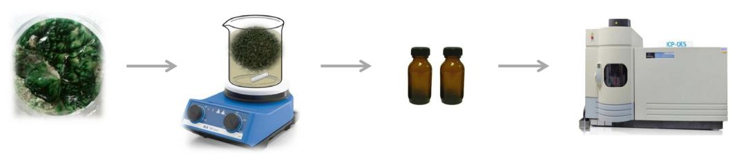
The algae washed and dried at 40 °C for 24 hours (constant weight). The biomass was sieved 0.85 mm. The solid to liquid ratio was 1 g dry wt./L.
