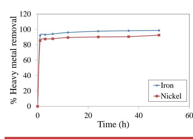
The optimum time of the metal removal from synthesis wastewater was 3 h. But the heavy metal removal rate from industrial wastewater will rise sharply in the first hour. This may be due to the presence of other elements in the industrial wastewater, which affects driving force and mass transfer resistance in the aqueous phase.
